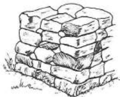
Weakly constructed end
